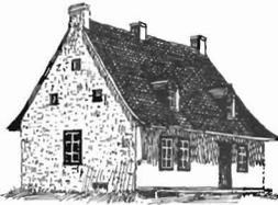
Triple chimneys, steep gable and bell-cast curve at the eaves (top) and multipaned casement windows are typical. Center chimneys (below) also are common.
