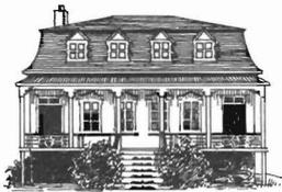
The mansard roof, the distinguishing feature of Second Empire style, here has a concave slope.
