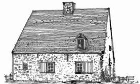
An early French type has a steep gable roof with no eaves trim. Hip-roof house (below) has slightly flared eaves.
