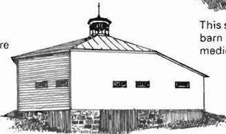
A central cupola tops a polygonal frame barn set on a stone foundation.
